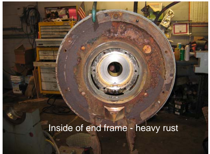
Rust on inside of end frame and machined fit
