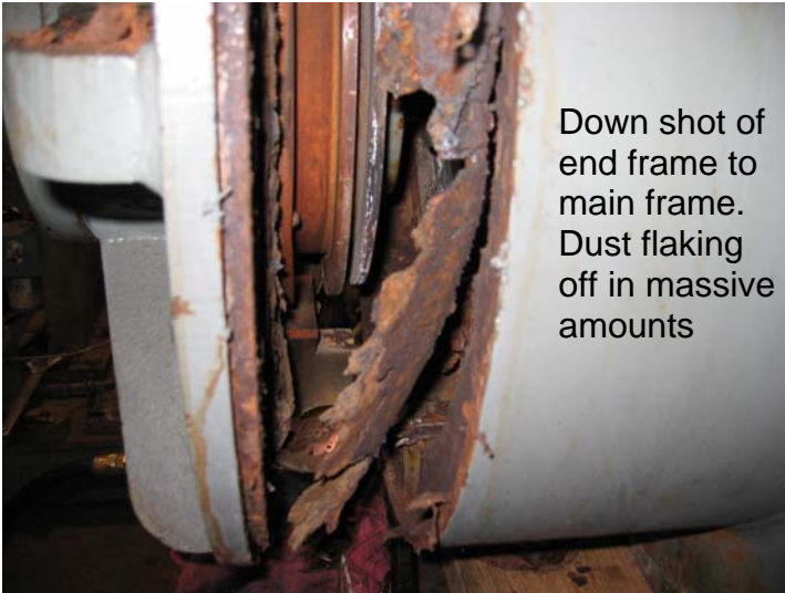
Rotor in spider frozen by rust - Over 6 tons to get apart
