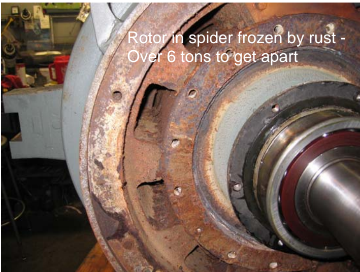
Rust on frame and machined fit
