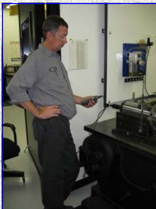
Install spindle in test stand and prepare for final test
