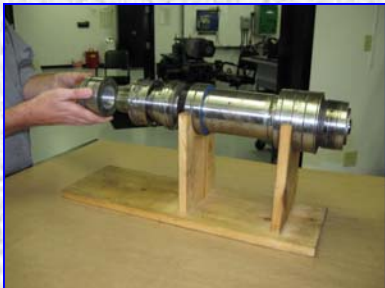
Dismantle starting at tail shaft, spider drive
