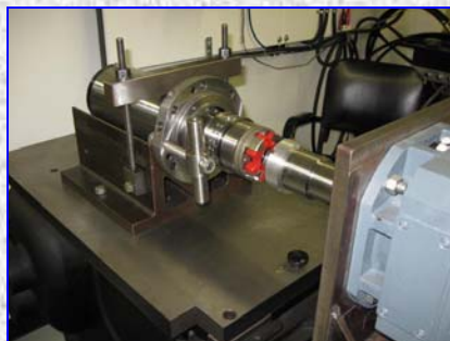
Test running in bearings, drawbar force, spindle taper accuracy and final trim balance
