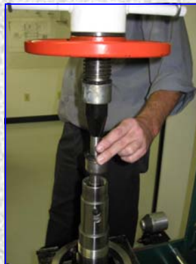
Continue dismantling at rear of spindle to gain access to bearing nut
