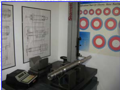
Before installing bearings test bar check for initial runout
