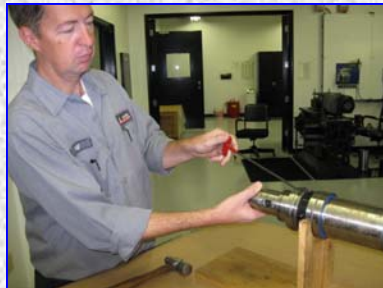
Continue dismantling at rear of spindle to gain access to bearing nut
