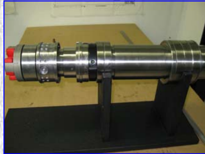
Final assembly stage before balance
