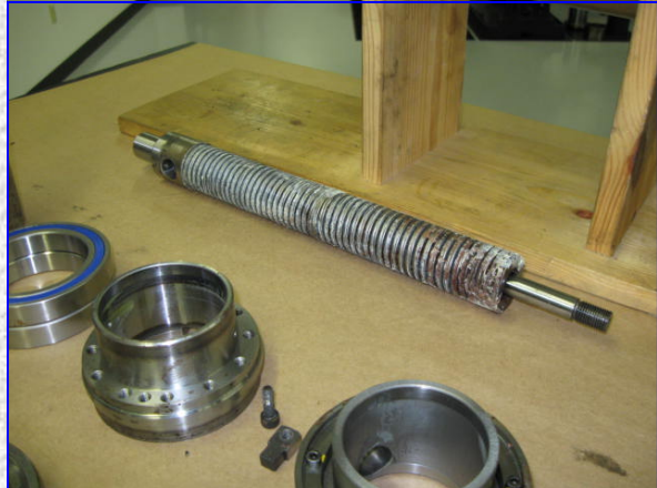
Inspect springs for cracks and wear and stack height
