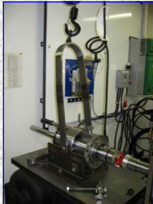
Install spindle in test stand and prepare for final test
