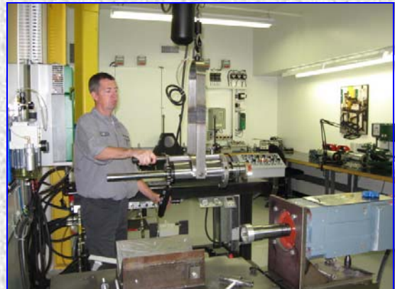
Install spindle in test stand and prepare for final test
