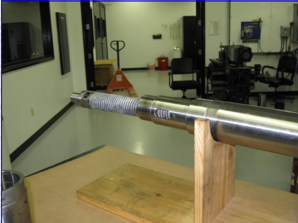
Inspect springs for cracks and wear and stack height
