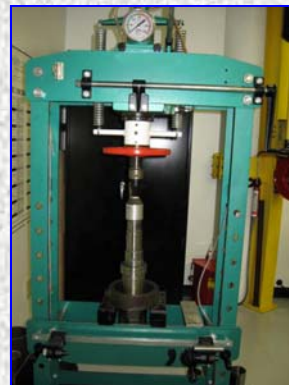
Prepare to remove drawbar, spring assembly and bearings
