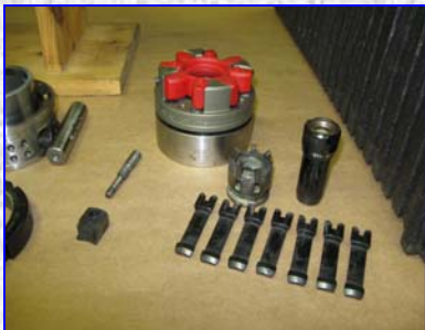
Inspect all disassembled components for wear and cracks
