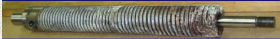
Inspect springs for cracks and wear and stack height
