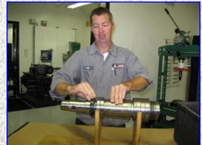
Remove bearing retainer nut
