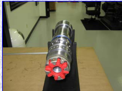
After balance, spindle is ready for final testing
